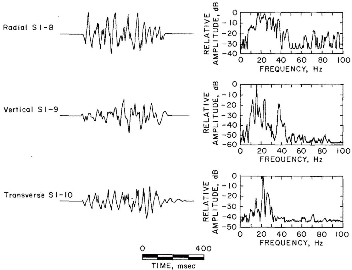
FIGURE 8. - Typical quarry blast vibration time histories.
