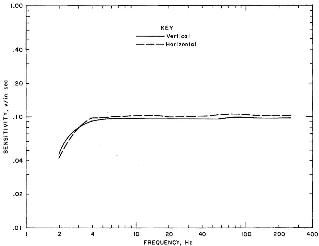
FIGURE A-20. - Vibra-Metrics model MB-120 sensitivity versus frequency.
