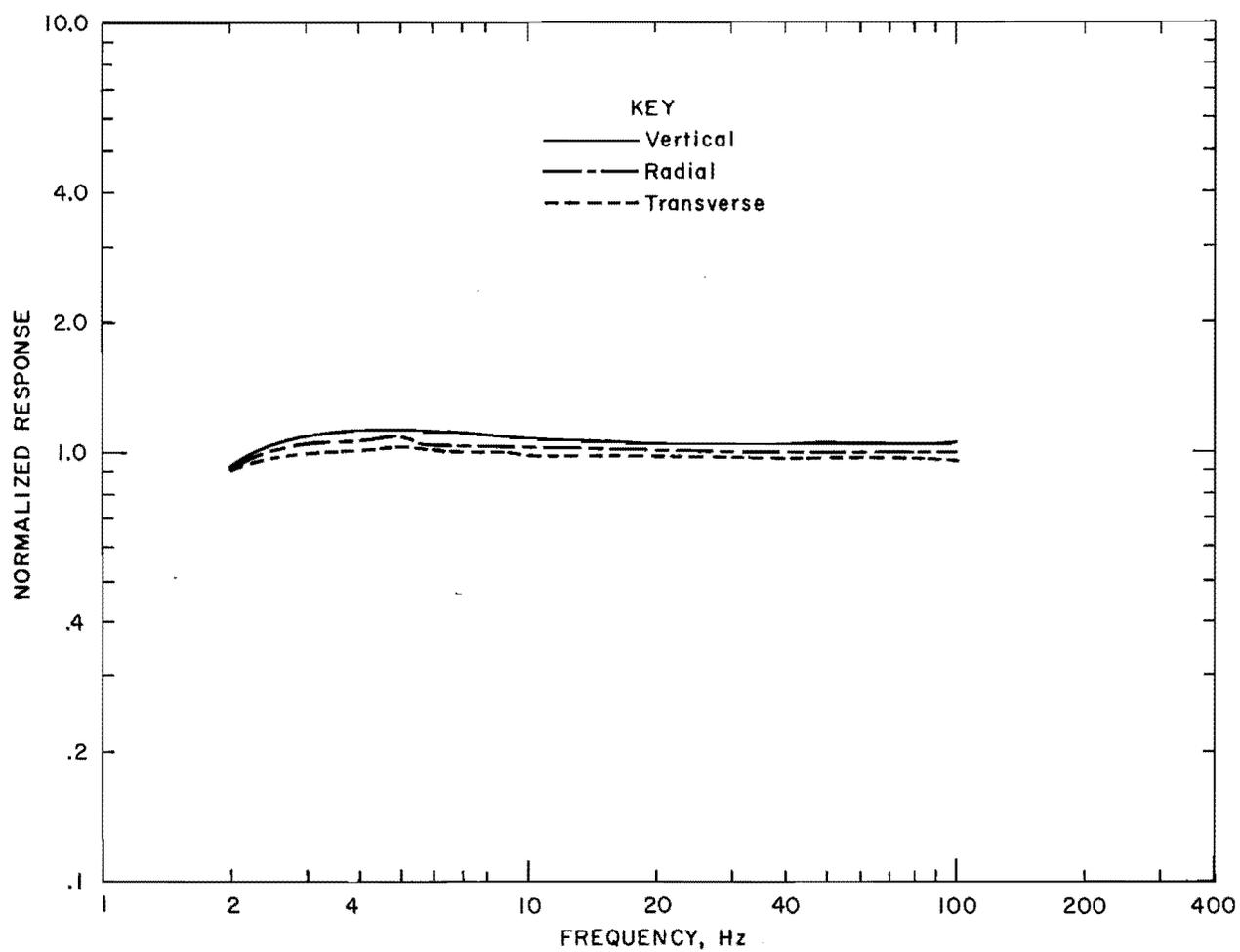
FIGURE A-4. - Dallas Instruments, Inc., model 3B-2 normalized response versus frequency.
