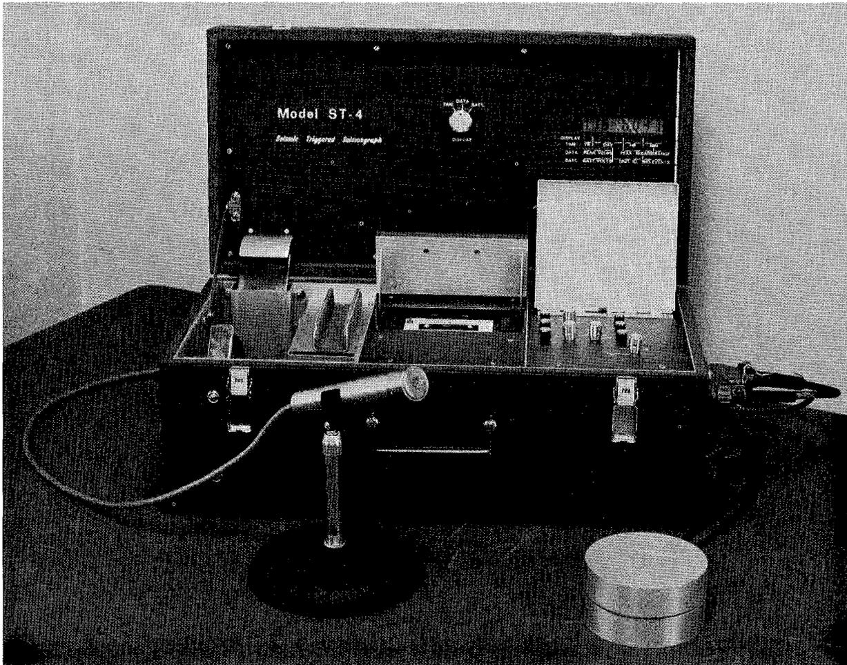
FIGURE A-5. - Dallas Instruments, Inc., model ST-4 seismic-triggered seismograph.
