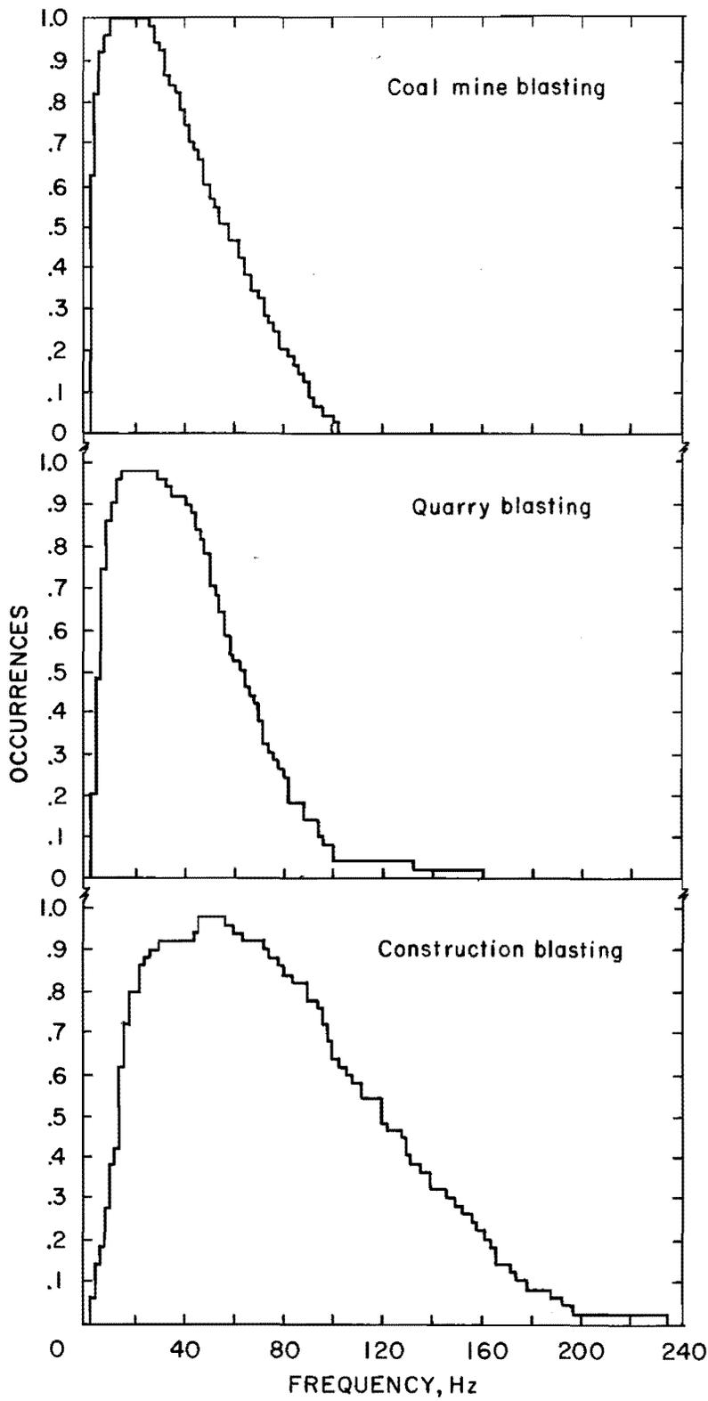
FIGURE 11. - Minus 20-dB-range histogram of coal quarry and construction blasts.
