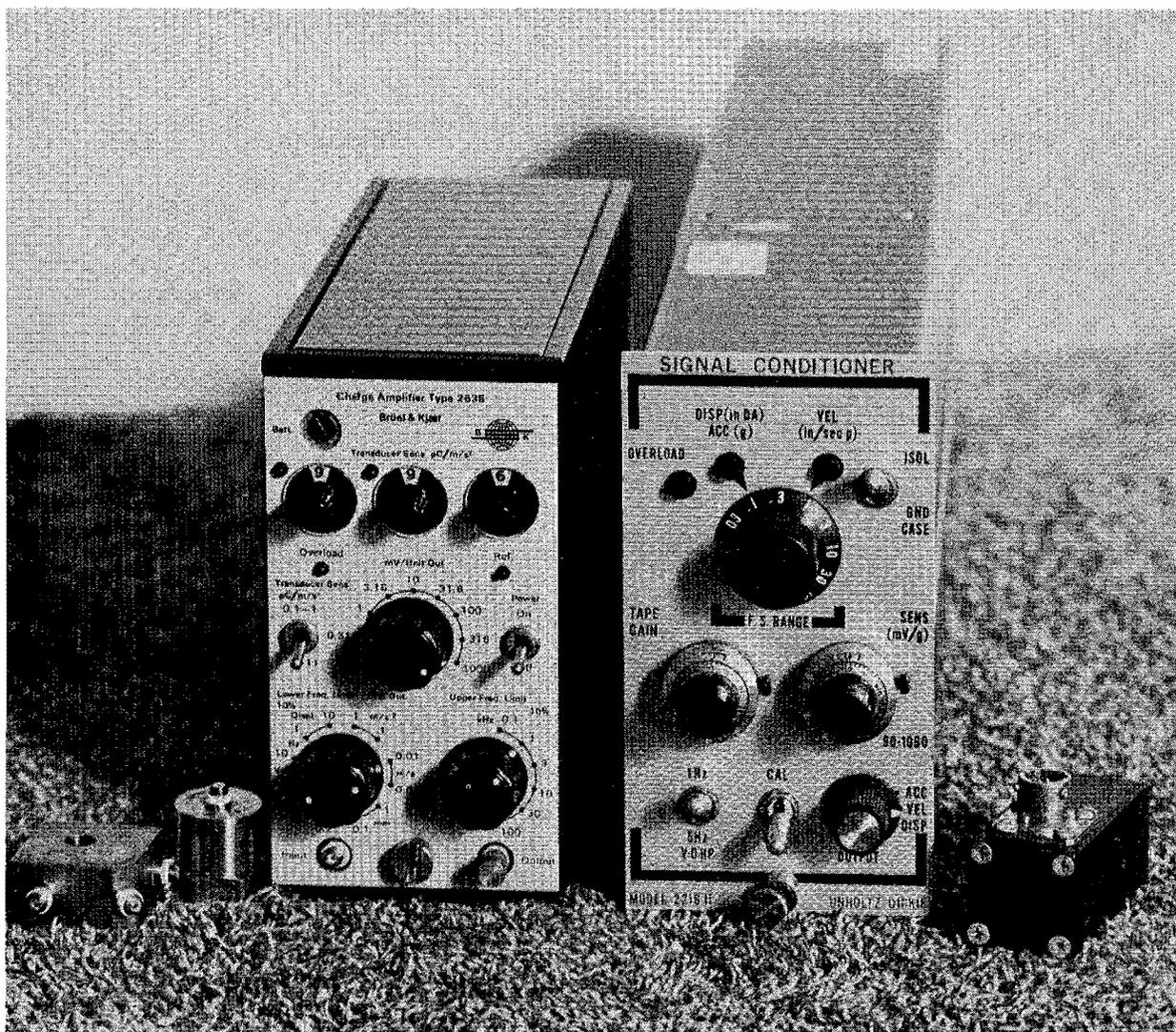
FIGURE A-28. - Unholtz-Dickie model 1000PA accelerometer and 221611 signal conditioner with B & K models 4370 and 4321 accelerometers and 2635 charge amplifier.
