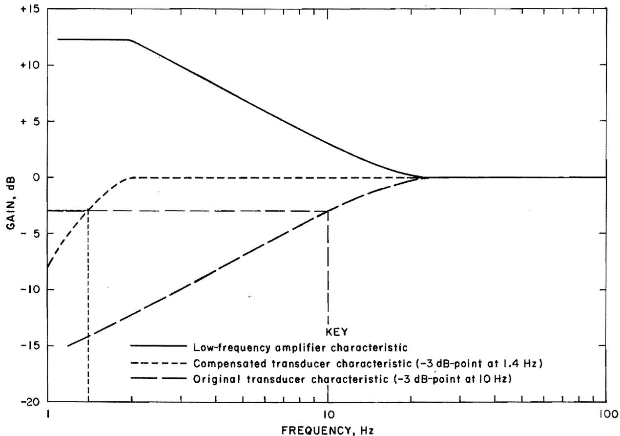
FIGURE 2. - Transducer low-frequency compensation.
