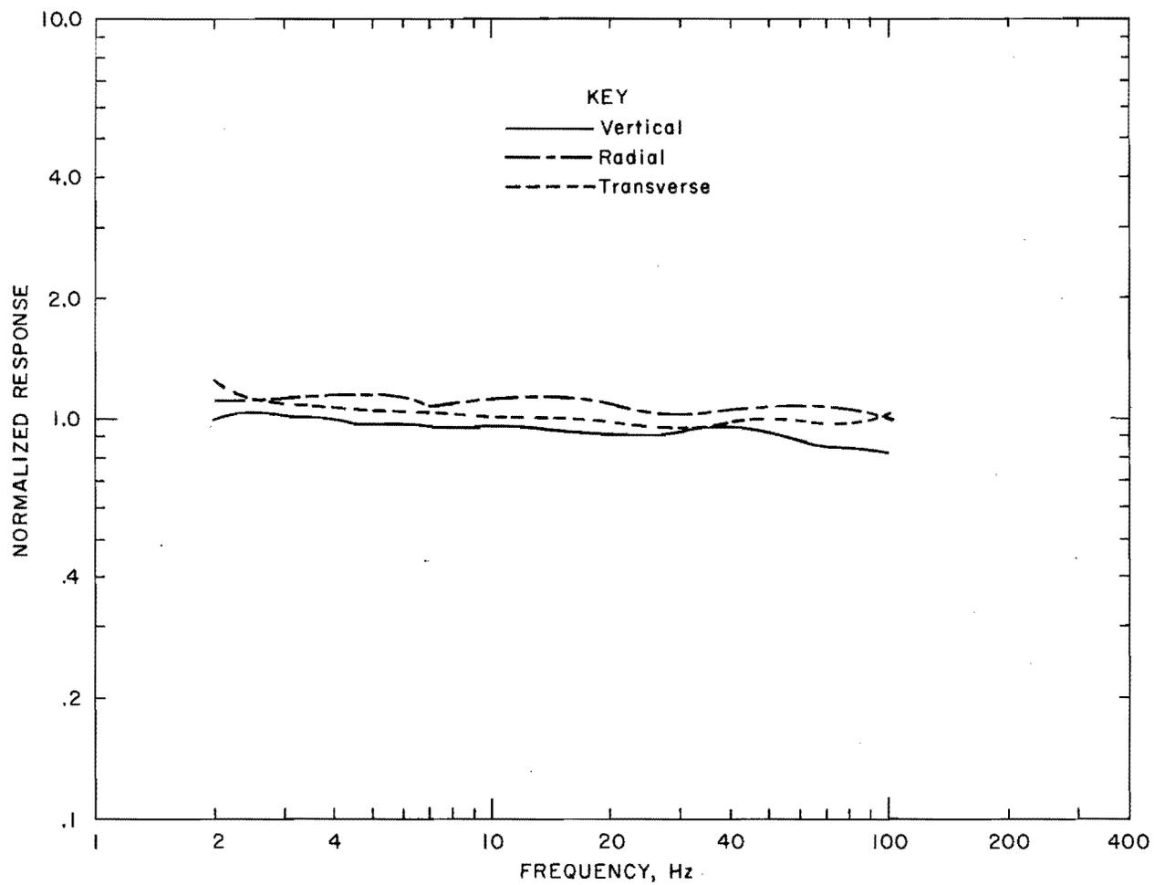
FIGURE A-12. - Vibra-Tech Engineers, Inc., model Vibra-Tape 2000 Series normalized response versus frequency.
