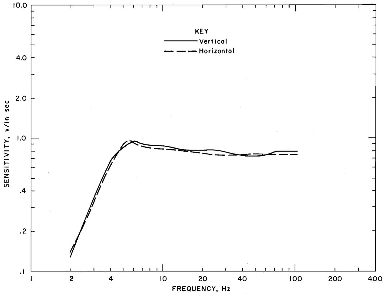
FIGURE A-26. - Mark Products model L-1B sensitivity versus frequency.
