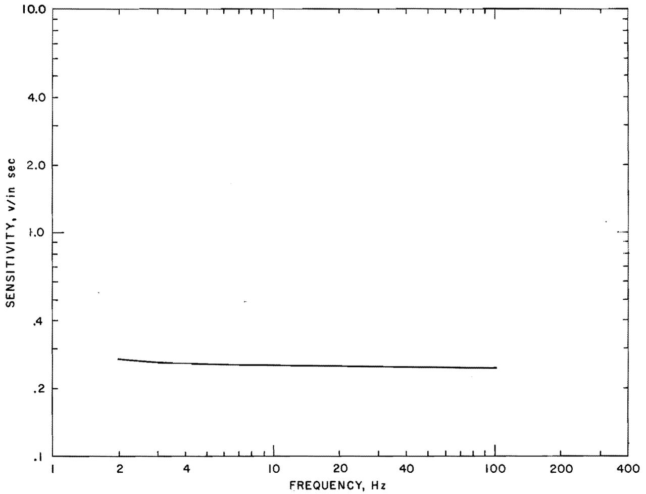
FIGURE A-30. - B & K model 4370 sensitivity versus frequency.
