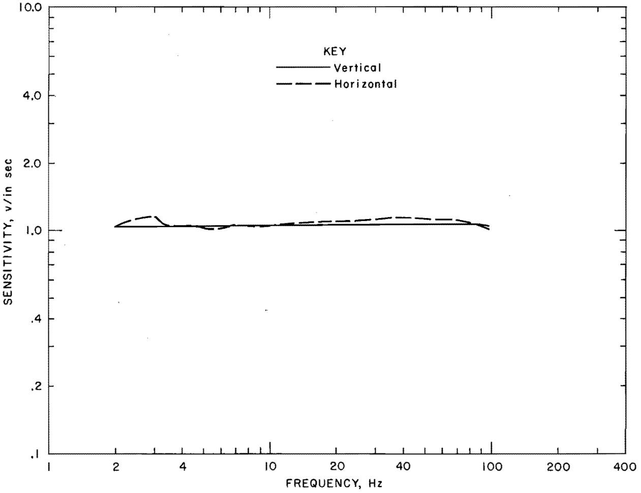
FIGURE A-29. - Unholtz-Dickie model 1000PA sensitivity versus frequency.
