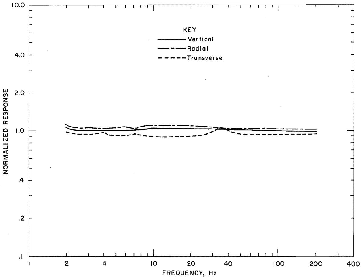
FIGURE A-6. - Dallas Instruments, Inc., model ST-4 normalized response versus frequency.
