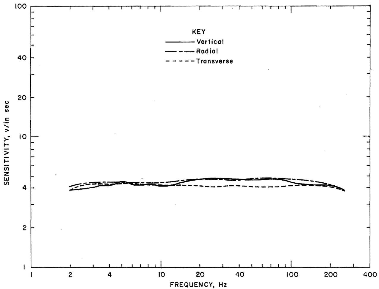
FIGURE A-24. - Geo Space triaxial model VLF-LP-3D sensitivity versus frequency.
