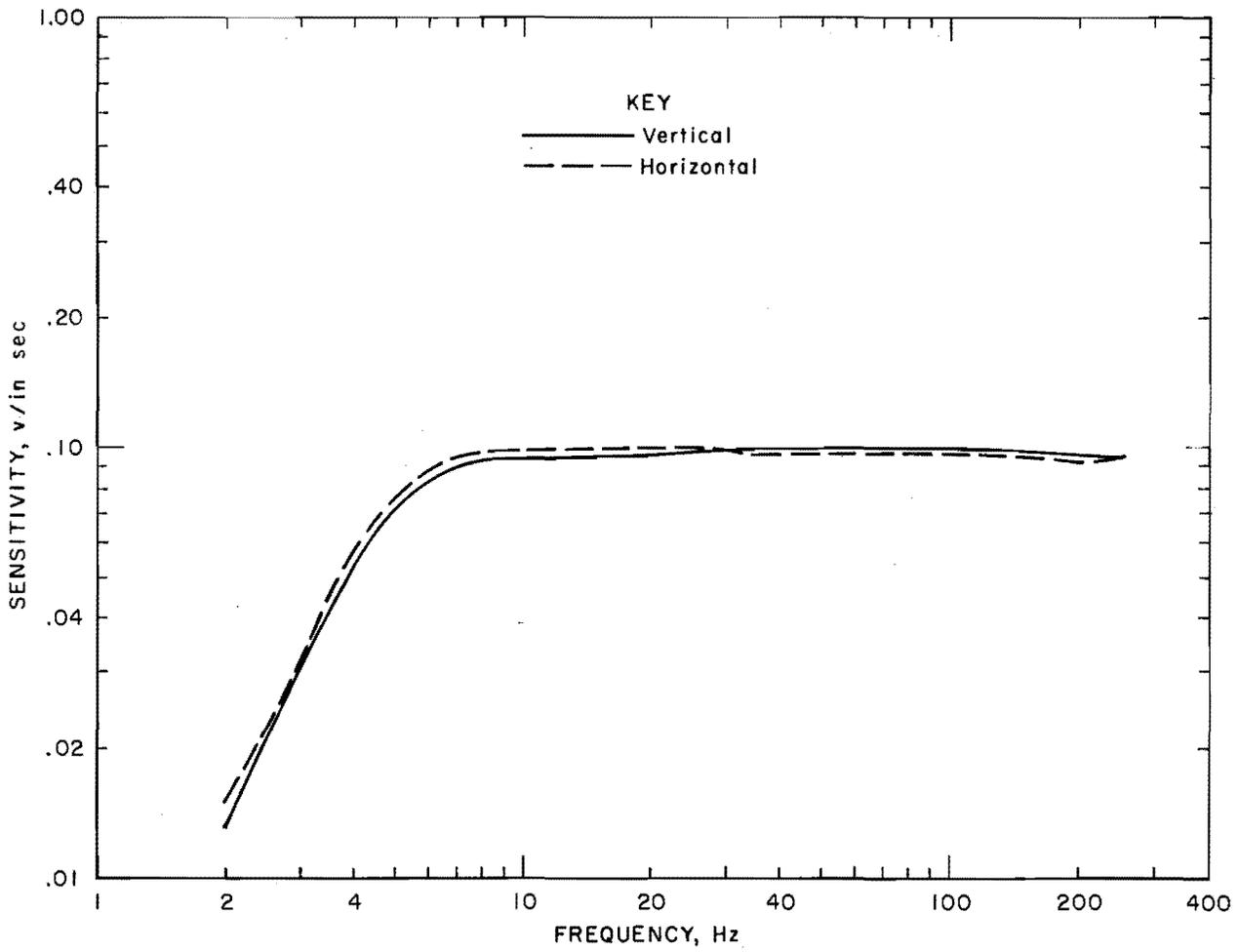
FIGURE A-21. - Vibra-Metrics model MB-124 sensitivity versus frequency.
