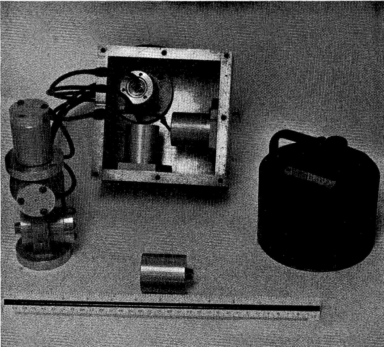
FIGURE A-22. - Geo Space models HS-1 and triaxial VLF-LP-3D velocity transducers.
