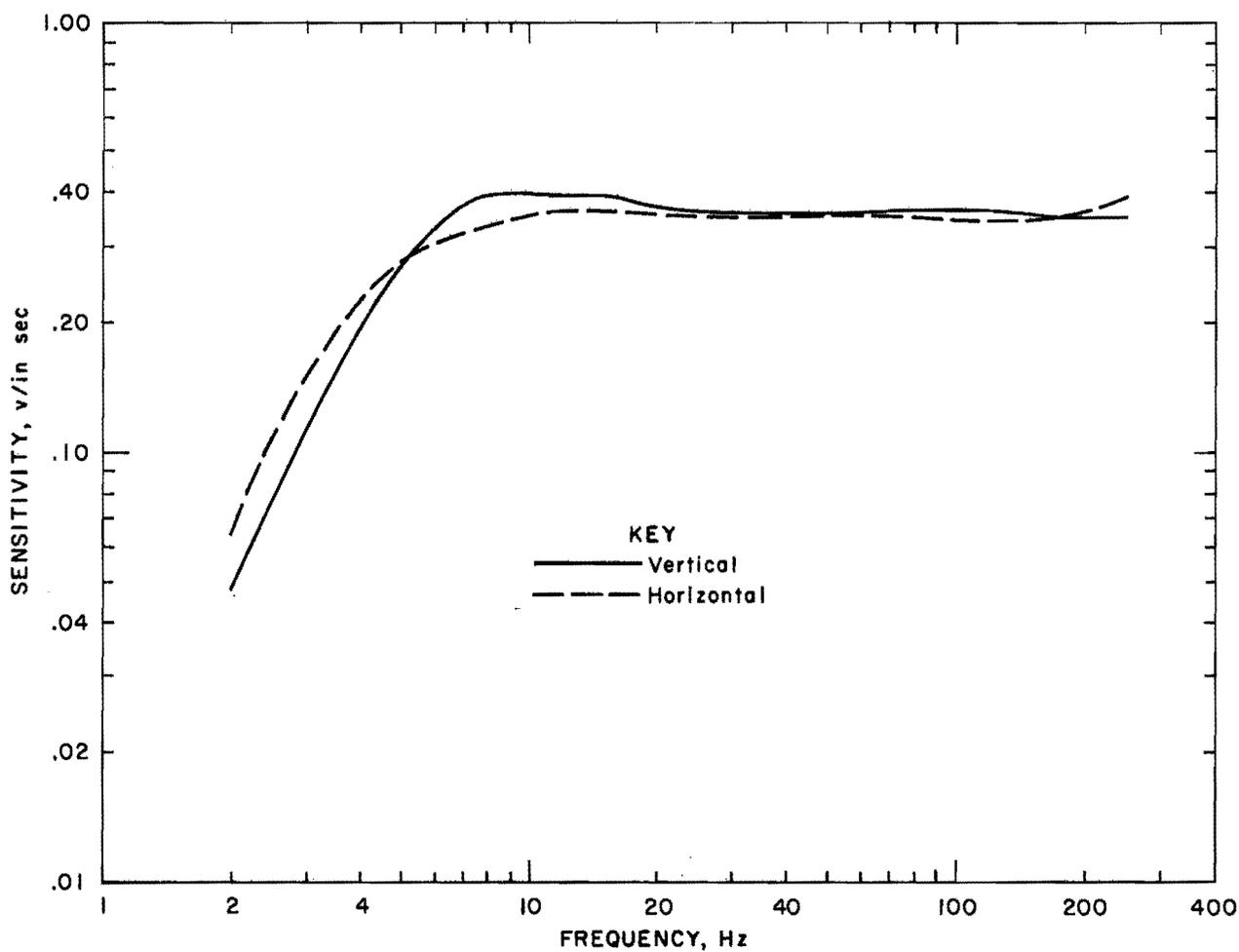
FIGURE A-23. - Geo Space model HS-1 sensitivity versus frequency.
