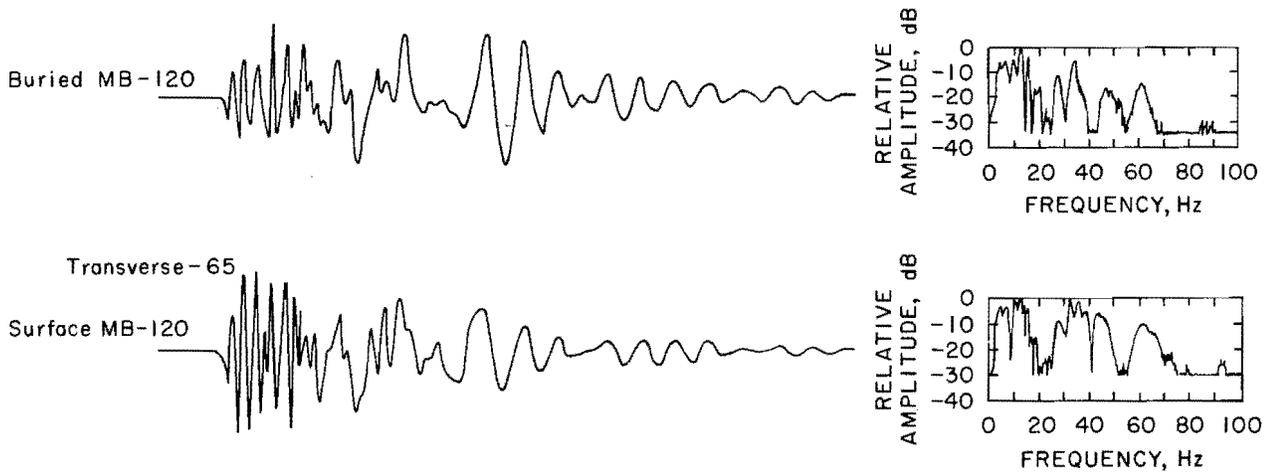
FIGURE 13. - Comparison of buried versus surface-placed transducer time histories.
