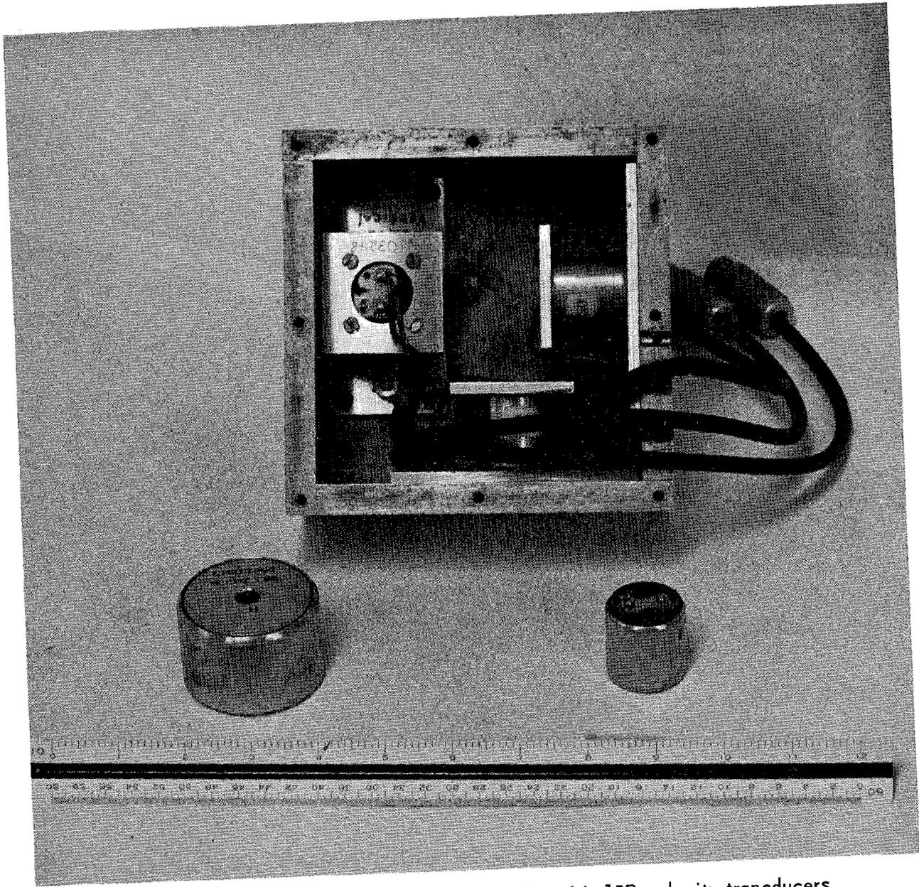
FIGURE A-25. - Mark Products models L-1B and L-15B velocity transducers.
