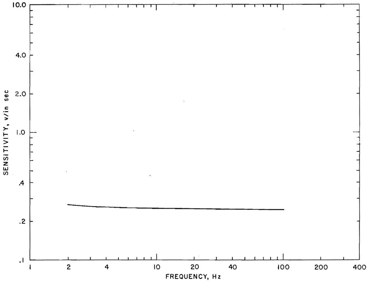
FIGURE A-31. - B & K model 4321 sensitivity versus frequency.
