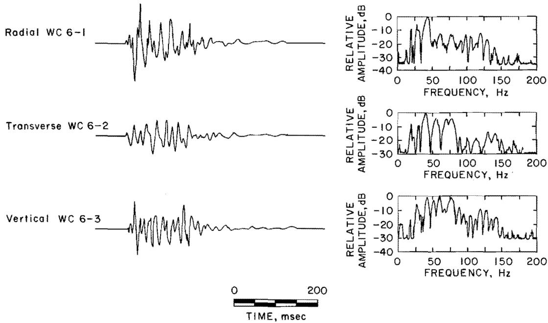
FIGURE 9. - Typical construction blast vibration time histories.
