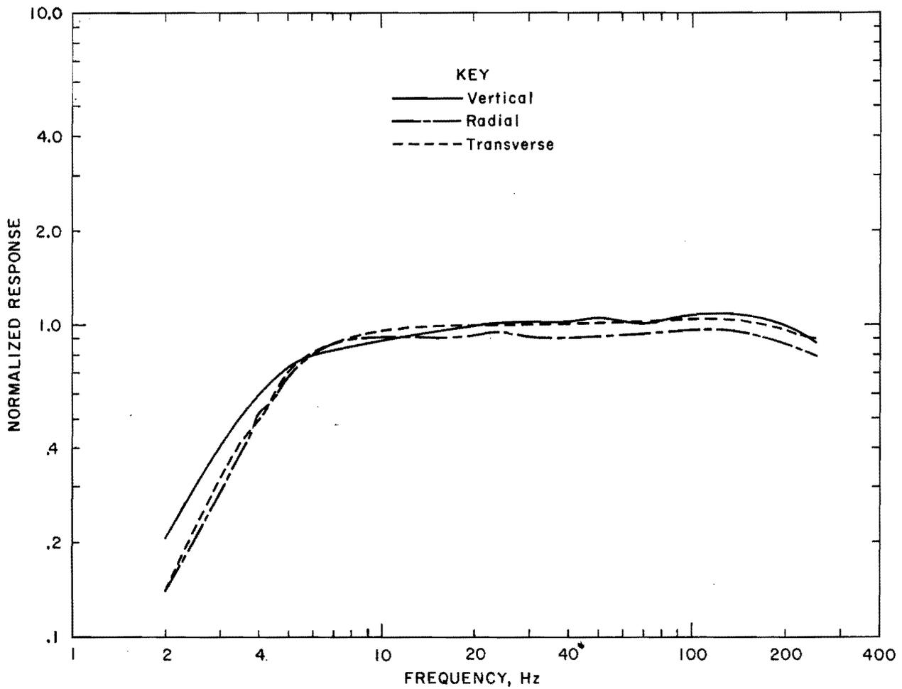
FIGURE A-16. - Philip R. Burger & Associates, Inc., model Seismic Safeguard Unit II normalized response versus frequency.
