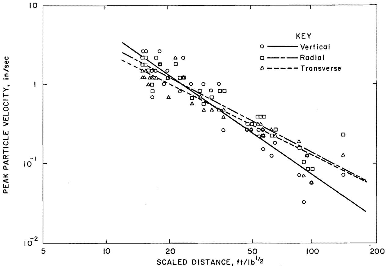
FIGURE 12. - Radial, transverse, and vertical particle velocity versus square root scaled distance.
