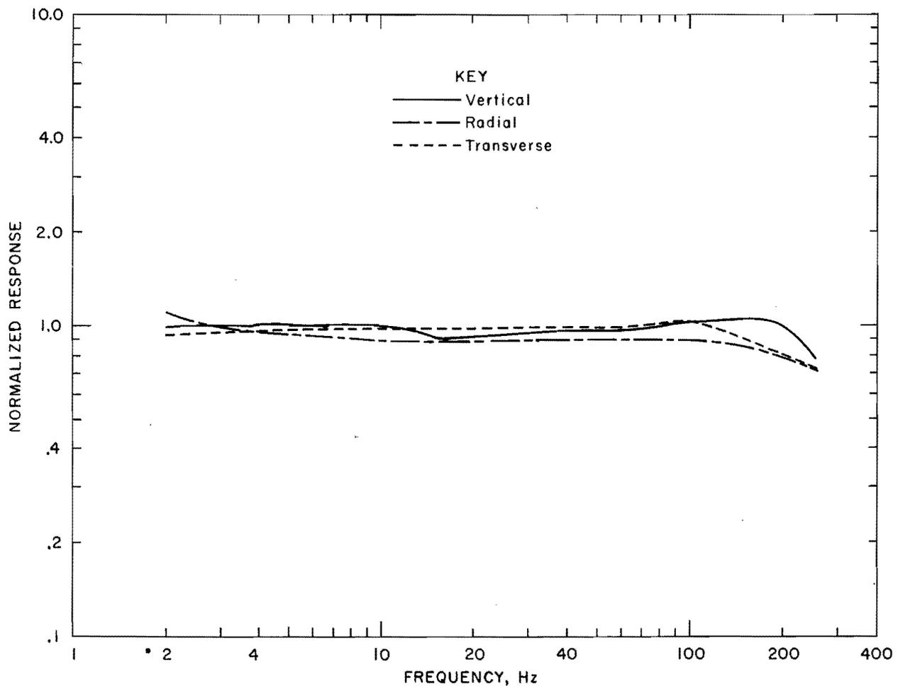
FIGURE A-2. - Dallas Instruments, Inc., model VS-3 normalized response versus frequency.
