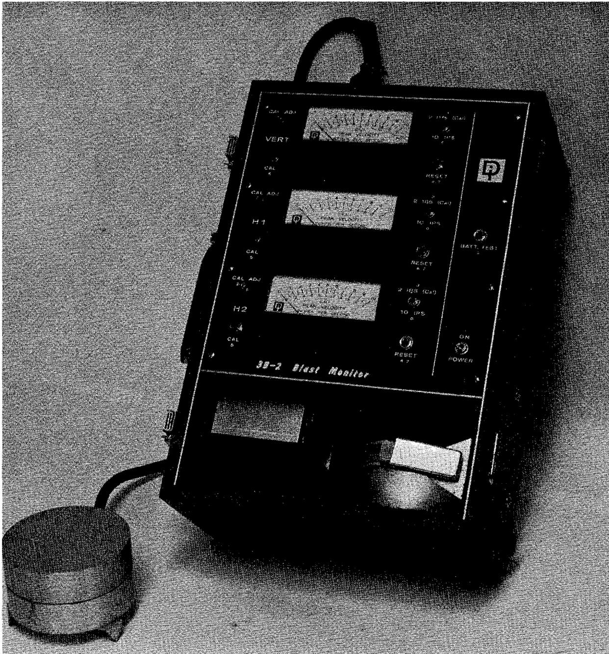
FIGURE A-3. - Dallas Instruments, Inc., model 3B-2 blast monitor.
