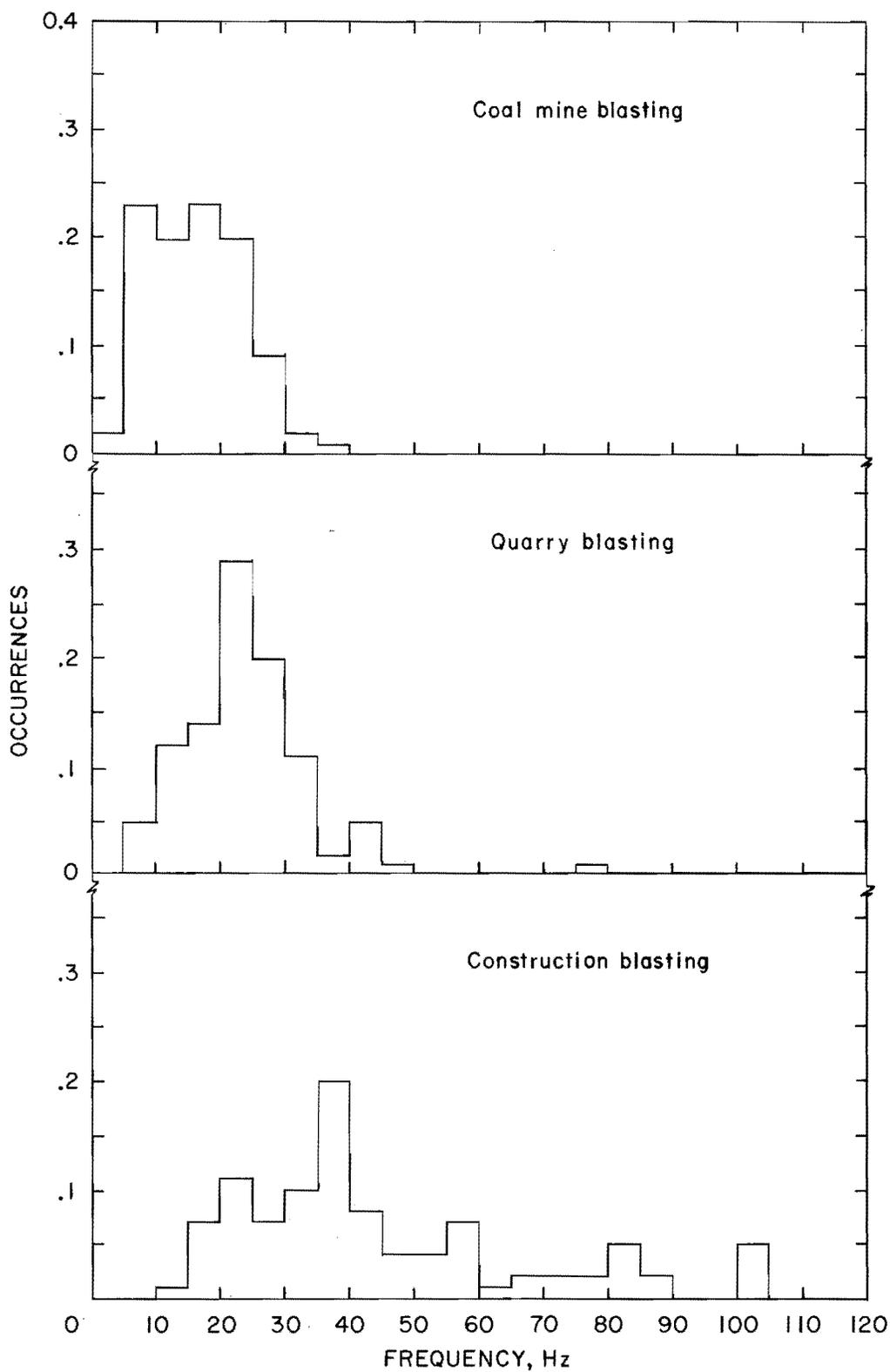
FIGURE 10. - Predominant frequency histogram of coal quarry and construction blasts.
