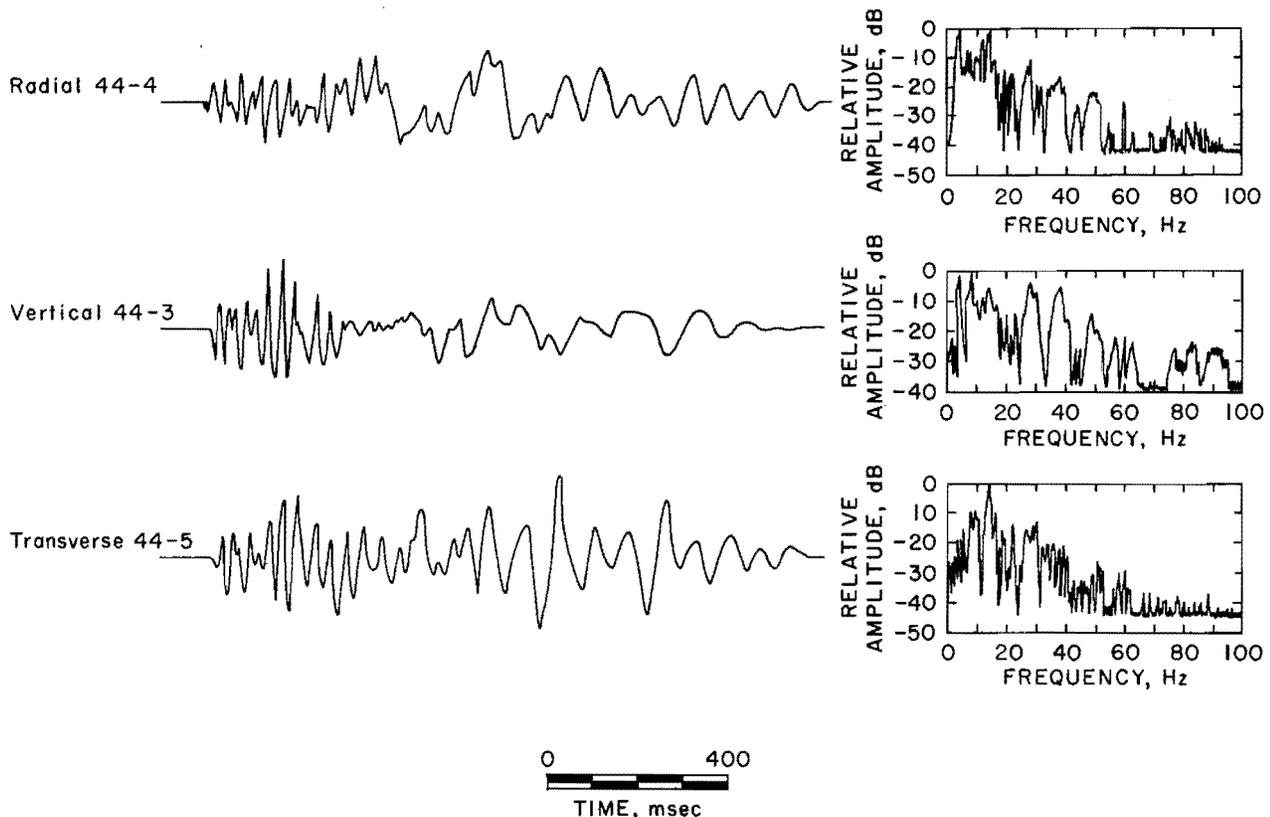
FIGURE 7. - Typical coal mine blast vibration time histories.
