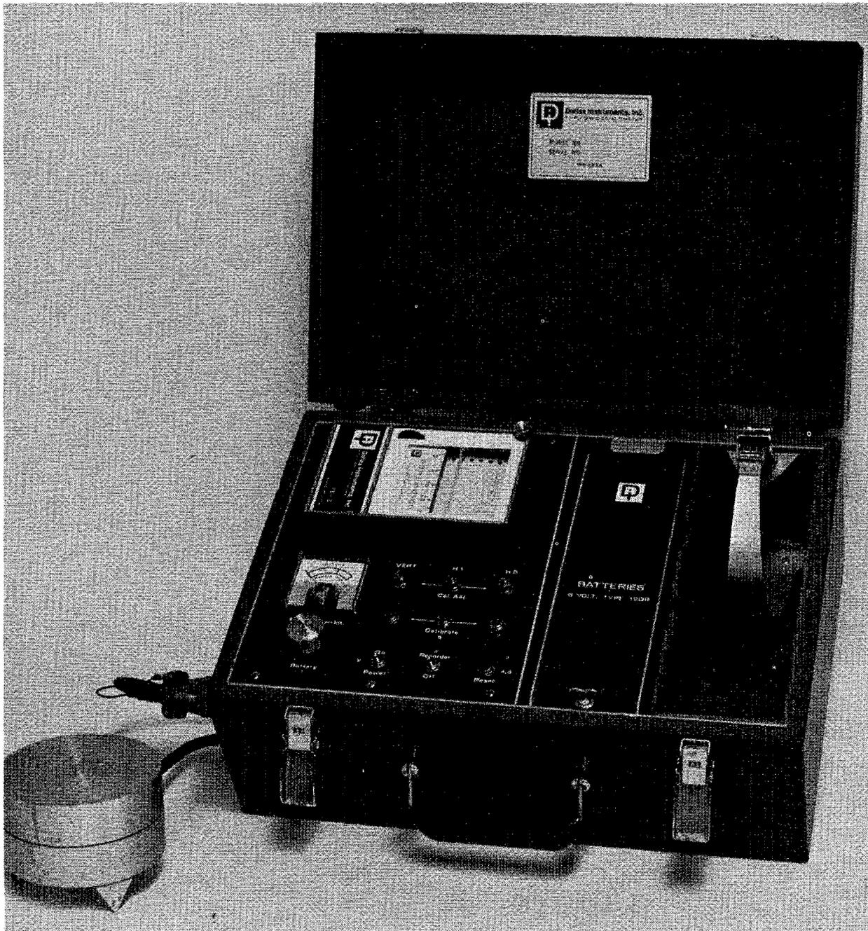
FIGURE A-1. - Dallas Instruments, Inc., model VS-3 blast monitor.
