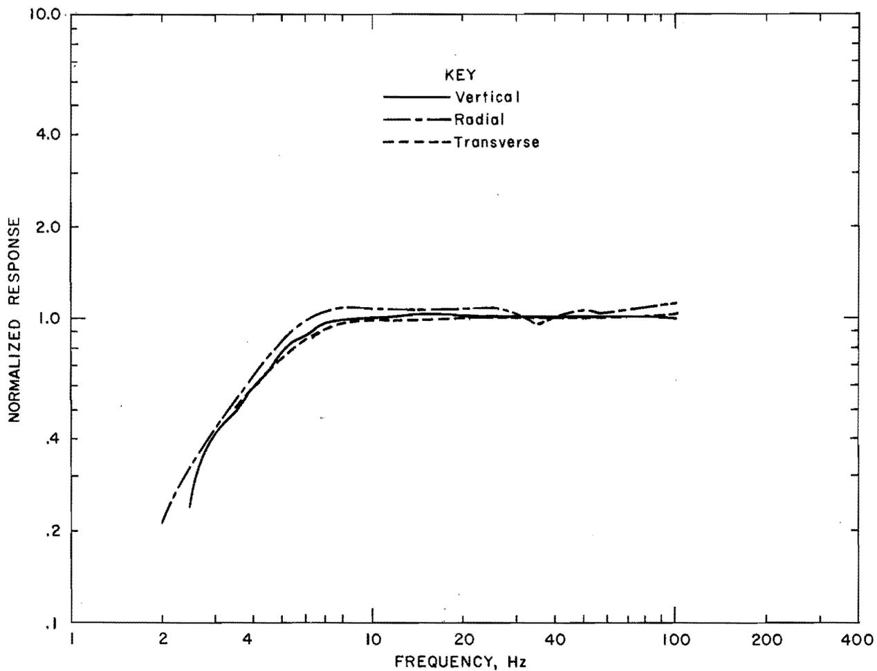
FIGURE A-8. - SINCO Slope Indicator Co., model S-4 normalized response versus frequency.
