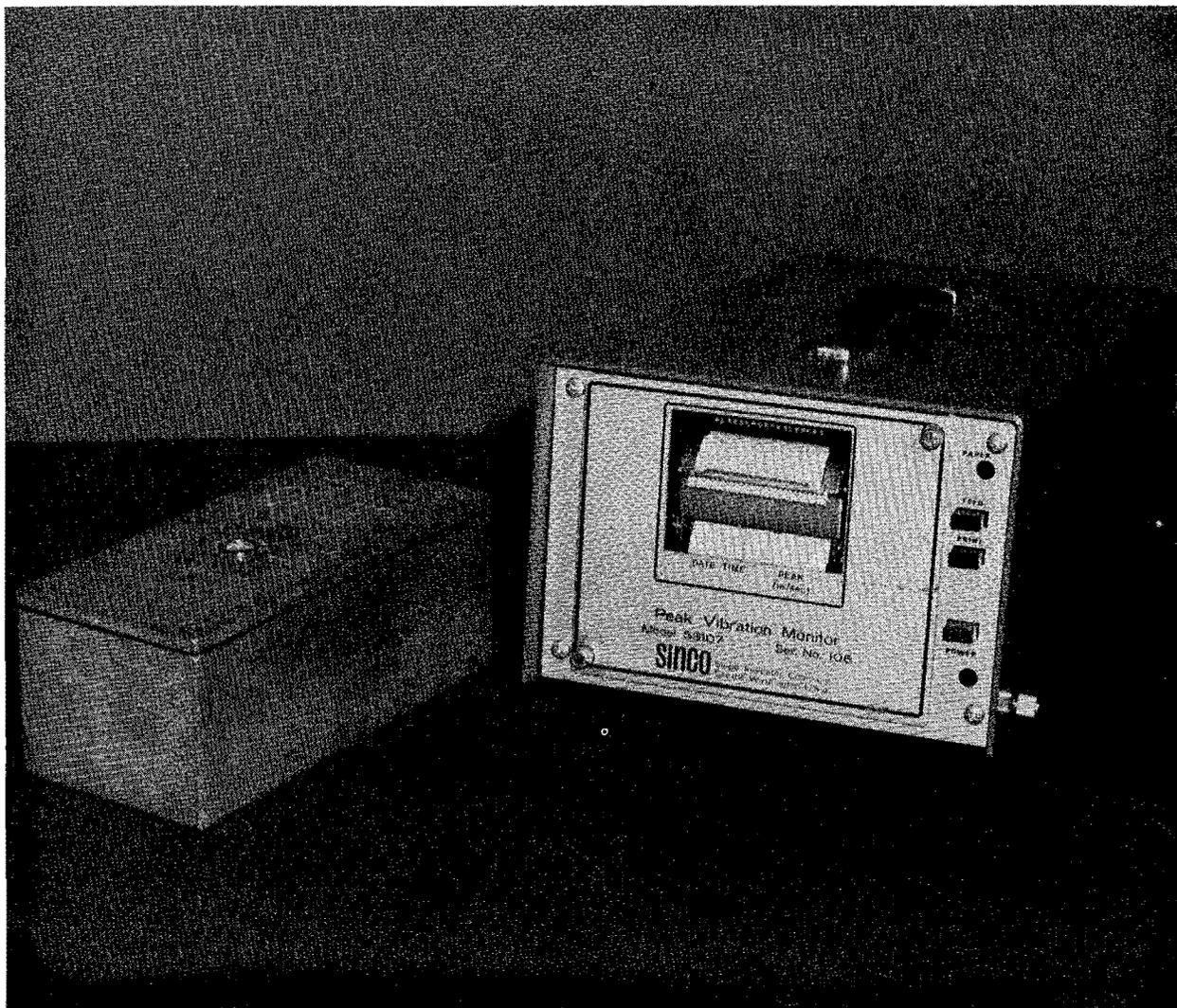
FIGURE A-7. - SINCO Slope Indicator Co., model S-4 peak vibration monitor.
