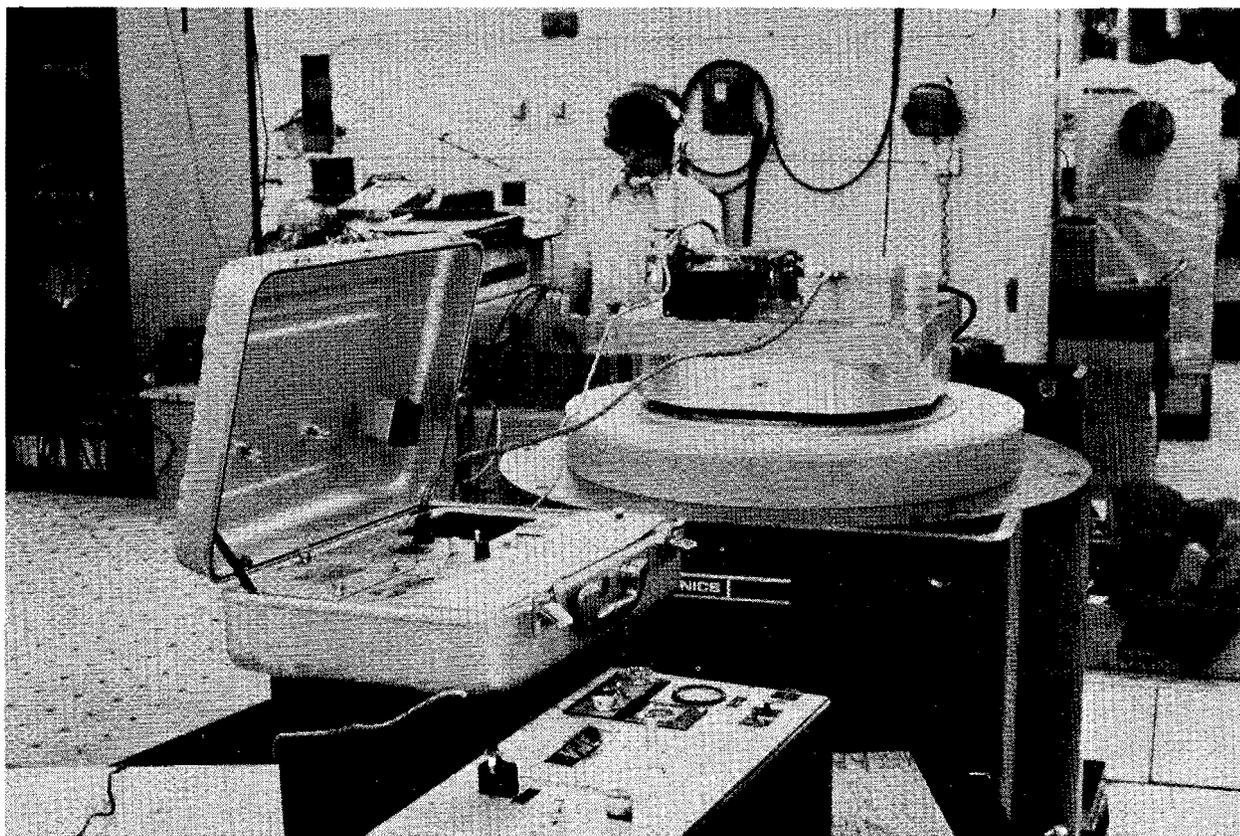
FIGURE 4. - U.S. Naval Research Laboratory shaker system.
