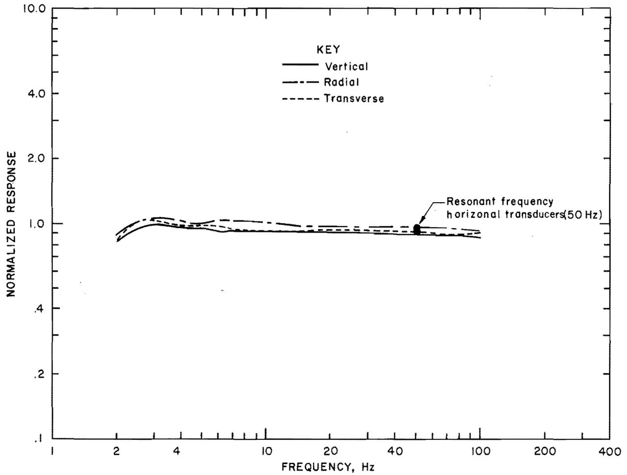
FIGURE A-18. - W. F. Sprengnether Instrument Co., Inc., model VS-1100 normalized response versus frequency.
