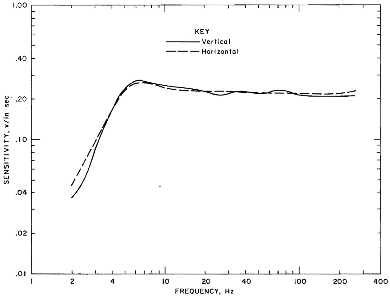
FIGURE A-27. - Mark Products model L-15B sensitivity versus frequency.
