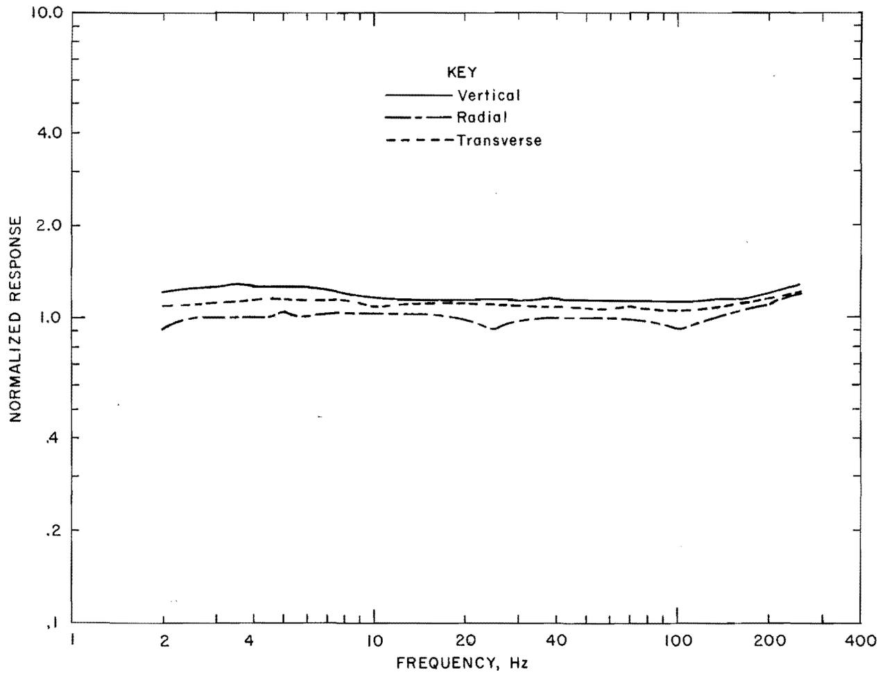
FIGURE A-10. - Vibra-Tech Engineers, Inc., model Vibra-Tape 1000 Series normalized response versus frequency.
