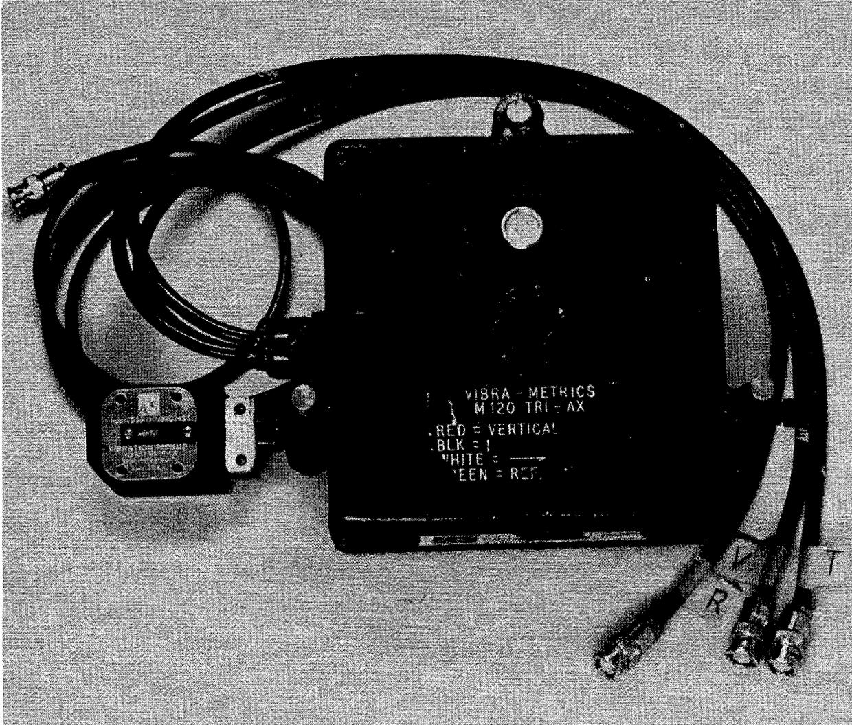
FIGURE A-19. - Vibra-Metrics model MB-120 transducer and triaxial box.
